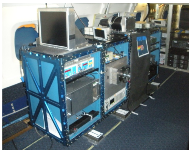
Figure 5-19 Photograph of the MFLL lidar mounted inside the NASA DC-8 aircraft.
