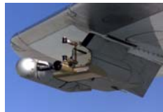
Wingtip probe used to measure aerosol and cloud particle size distributions and cloud liquid water content.
